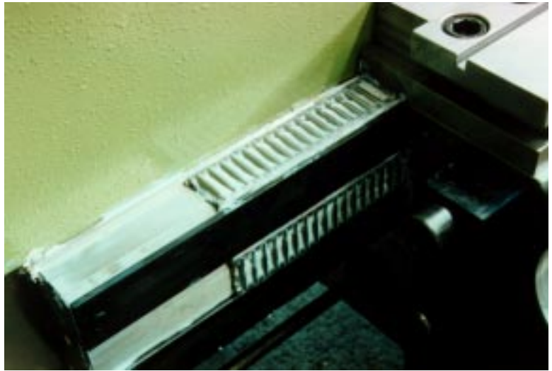
Cross slide mounted on vertical slide with pre-loaded pins slideways for the displacement of motor head in a transverse direction.
